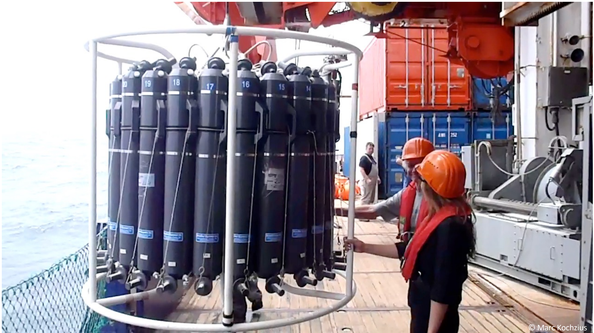
Rosette with CTD and Niskin bottles on RV Polarstern
