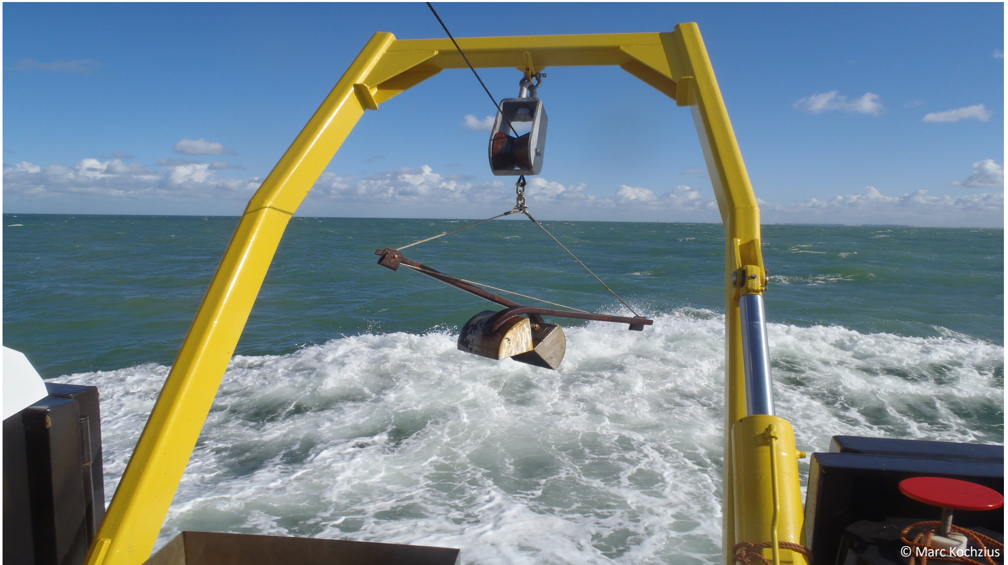
Van Ven grab for sediment samples
